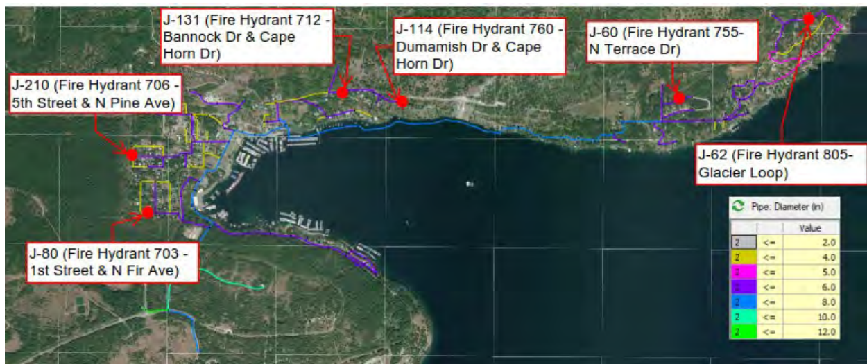
Figure 1 - Fire Flow Historic Test Locations
